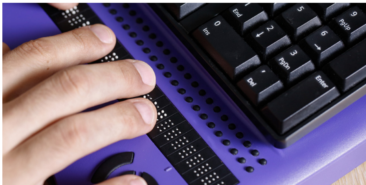
A Braille Display allows the visually impaired user to read the content of the document.
